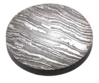
damascus steel layered from medium-carbon tool steel and low-carbon nickel steels, made cheaply in India, etched and hardened, but untempered 25,000 volts DC negative resonant pulse over Regent Royal orthographic film.
