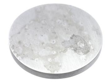
aluminium, the only sample to deteriorate through imaging, the applied voltage depositing very thin patches of aluminium splatter over the emulsion, as can be seen.... this is low quality matter 30,000 volts DC over Arista orthographic film.
