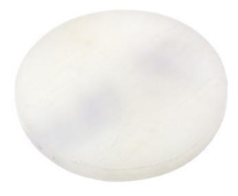
high density polyethylene from contemporary jeweller Mark, formed by fusing used milk containers into sheet under heat and pressure in his kitchen oven (the use-by-date ink shows through in embedded layers), to be used for making contemporary jewellery artwork stuff 10,000 volts AC at 2000Hz over Arista orthographic film.
